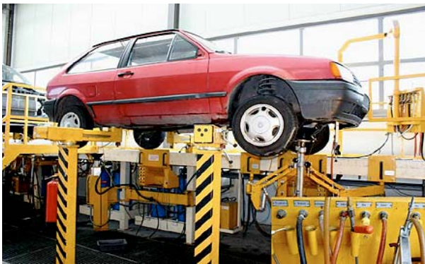
Drain of operating fluids
