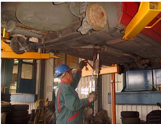
Dismantling of catalyst
