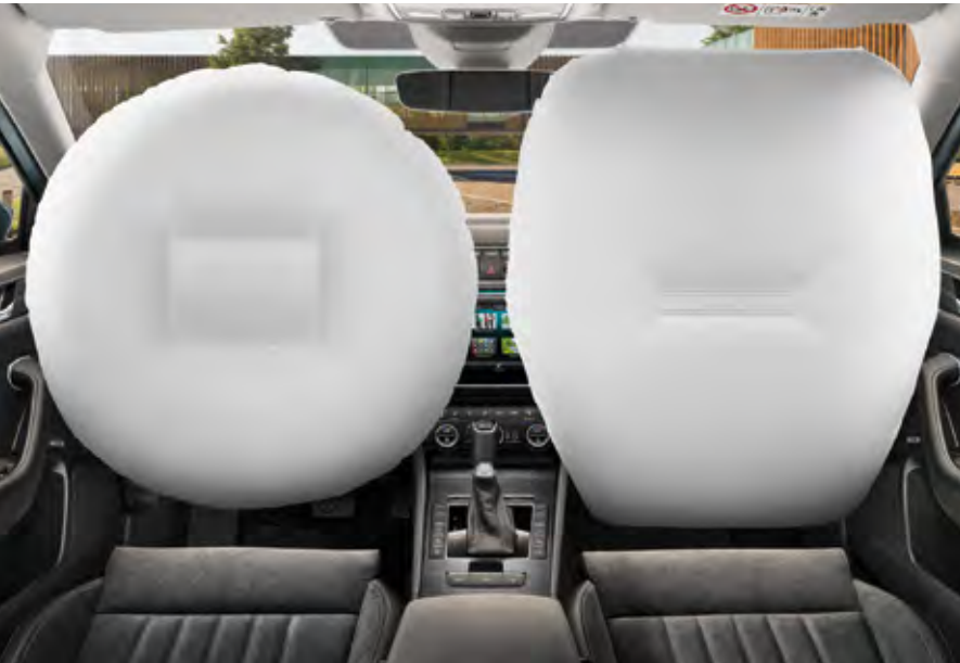
FRONT DRIVER AND PASSENGER AIRBAG While the driver airbag is enclosed in the steering wheel, the passenger airbag is located in the dashboard.
