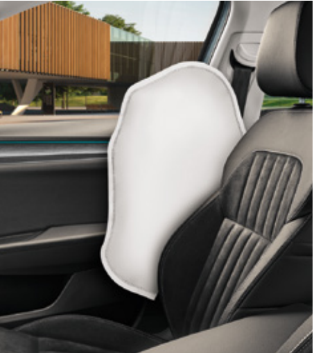
FRONT AND REAR SIDE AIRBAGS These four airbags protect the pelvis and chest of the driver and other passengers in the event of a side collision.
