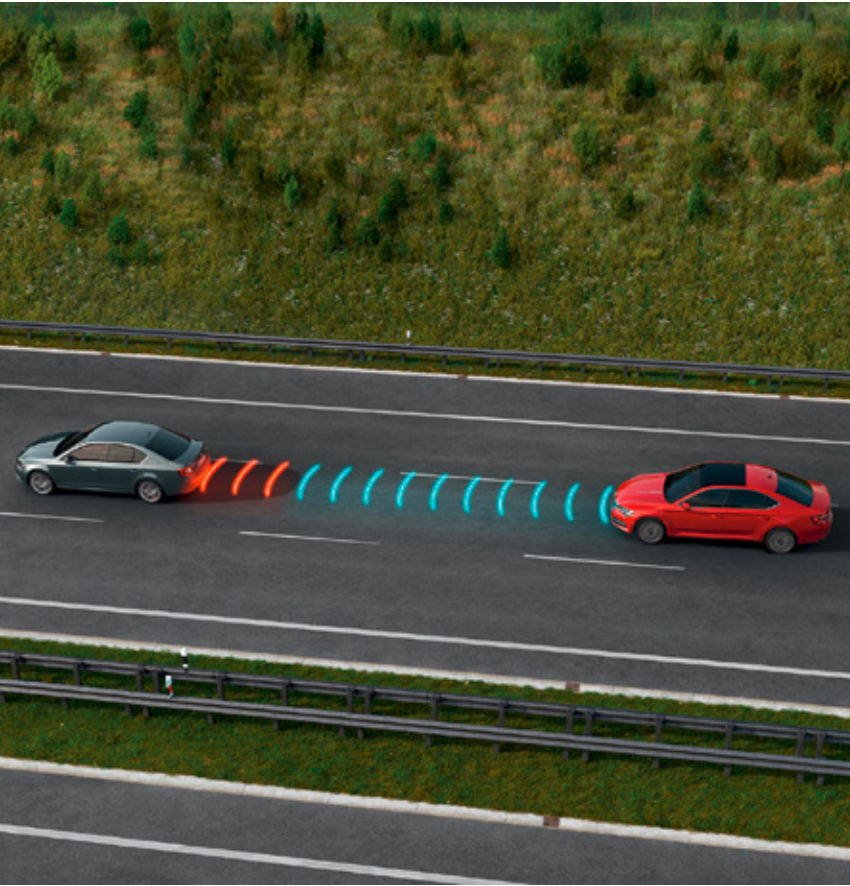
ADAPTIVE CRUISE CONTROL Using a radar device in the front grille, in addition to its basic cruise control function. This assistant system maintains a safe distance from vehicles in front of you to increase driver comfort while reducing fuel consumption and CO2 emissions.
