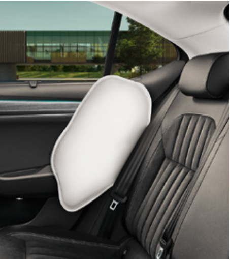
FRONT AND REAR SIDE AIRBAGS These four airbags protect the pelvis and chest of the driver and other passengers in the event of a side collision.
